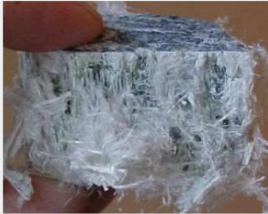
FIG-13 Asbestos fibers
